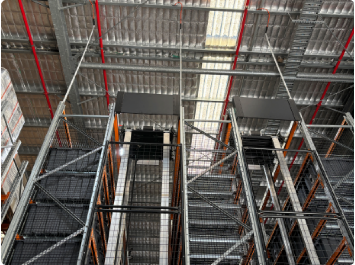
Example Installation with Three Rows of Racking and Two Shelfbots
