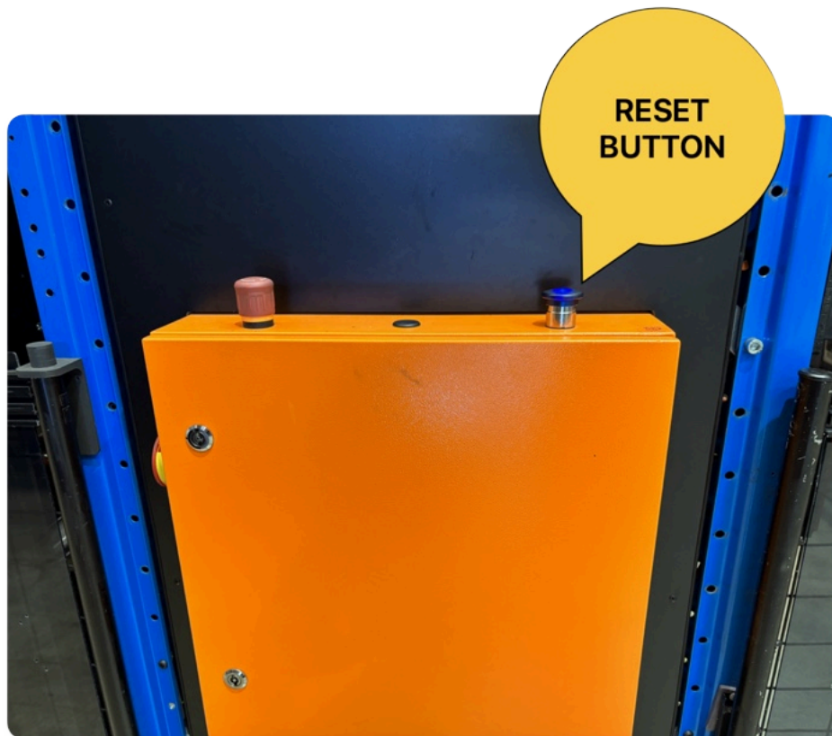
Blue Reset button installed on the top right side of the Safety Control cabinet
